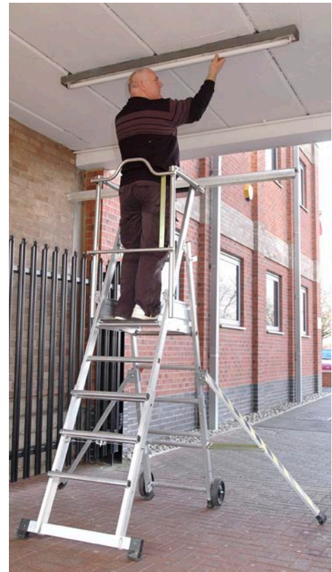
Figure 22 Working platform stepladder
