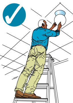
Figure 20b Correct – three clear steps
