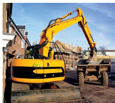
Figure 36 Minimal tail swing
